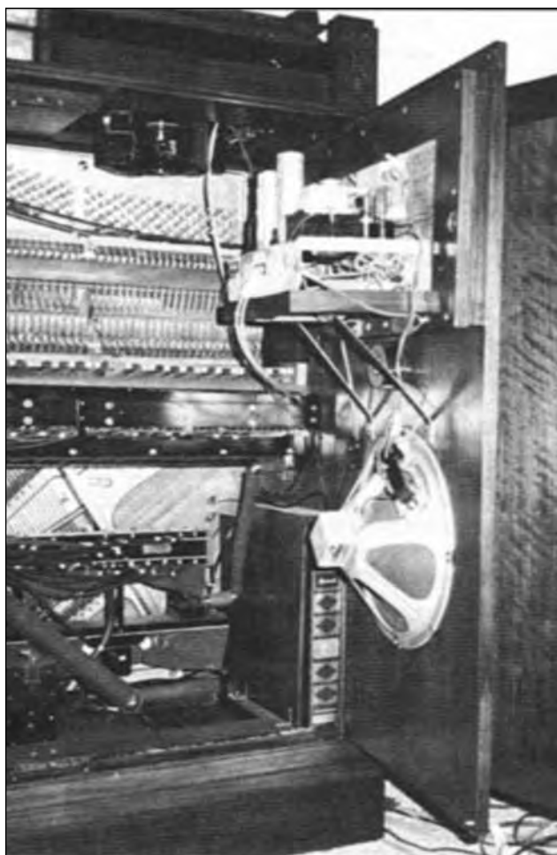
View of 12" speaker and tube chassis of RCA Radio/Amplifier for Phonograph.
