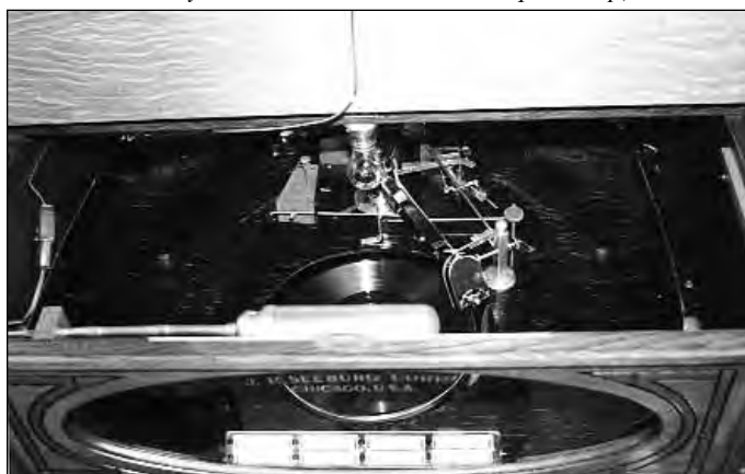
Turntable showing pneumatics used to move tone arm. (Electric lamp illuminated only when record is playing) (Title strip lamp is on continuously to attract attention, as is marquee lamp)
