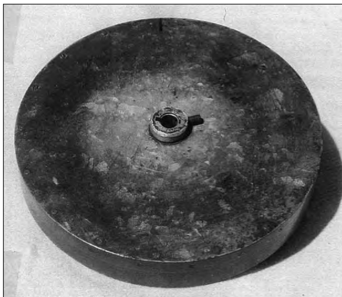
The copper band unit which drives the interrupter mechanism. Outside view.
