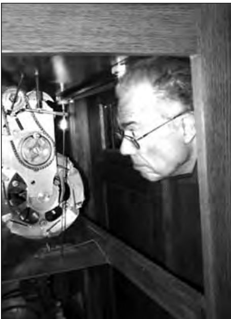
Dave Palter inspects the Wurlitzer roll changer through the front access door.
