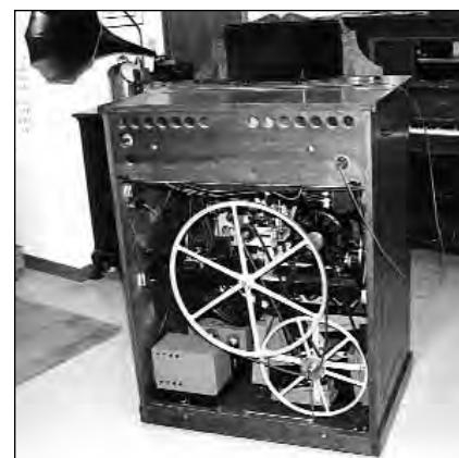
Rear view revealing electric motor (same type as in coin pianos) Small box type vacuum pump, "operadio" 5 tube (Triode Type) Amplifier, and valve block in upper right hand corner
