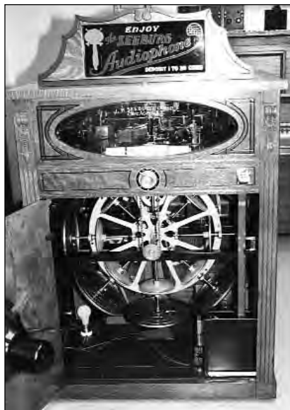
Front door open revealing "Ferris Wheel" of 8 turntables, coin box, and electric lamp used as a resistor in the coin accumulator circuit
