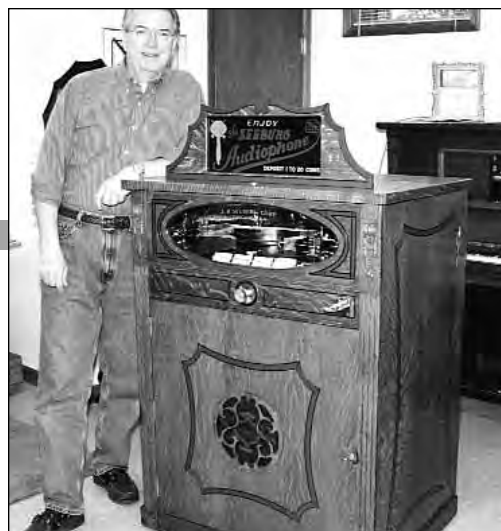
Front view with selector knob, title strip, coin slot (nickels only) and rear illuminated marquee.
