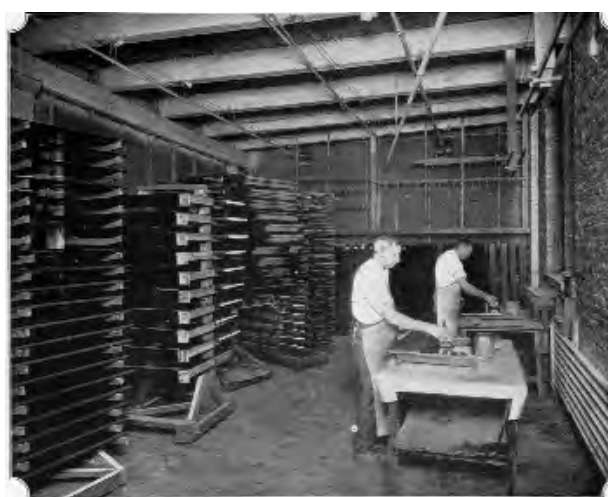
Staining panels and posts as part of case construction and finishing.
