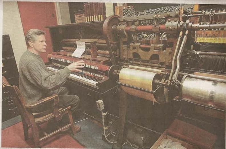
Bob Berkman, QRS music director and Buffalo office manager, explains the operation of the piano attached to the perforating machine that makes the master piano roll that other machines would then duplicate.
